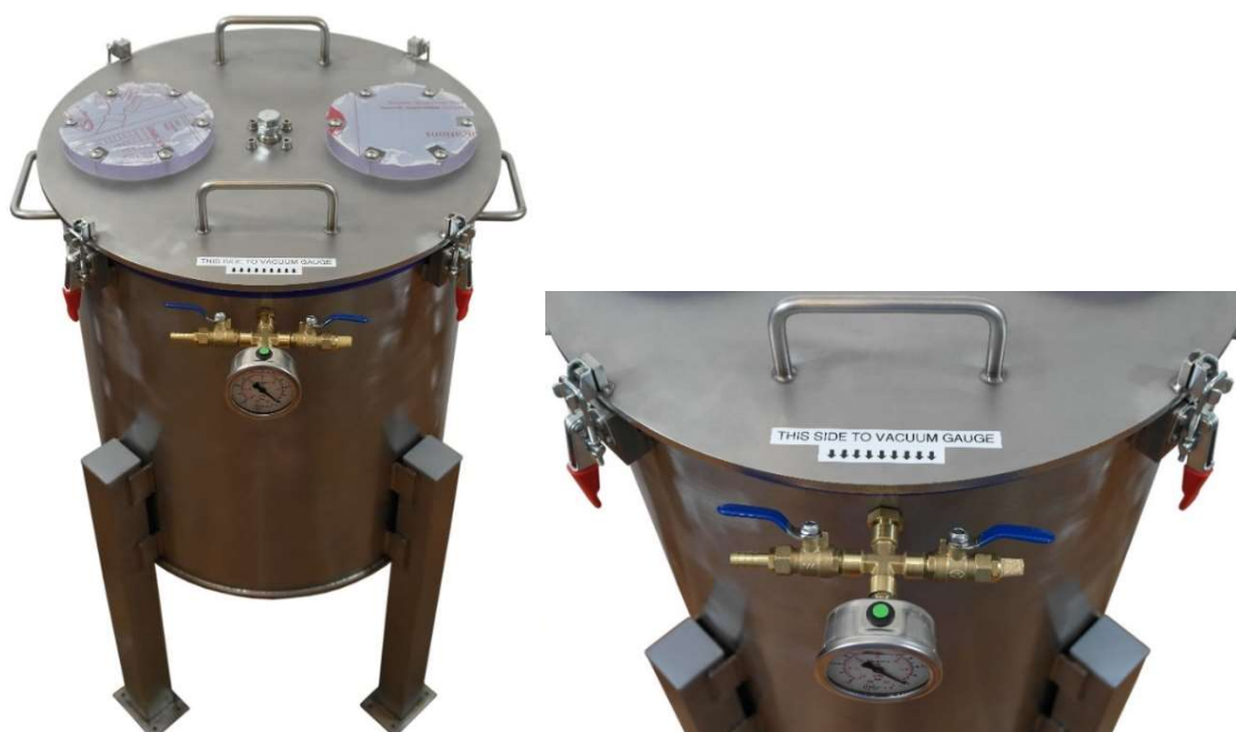
Photo 14: Correct location of the lid on the chamber.
