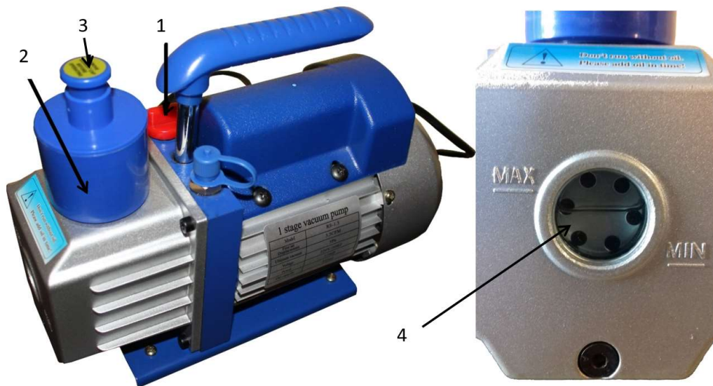
Photo 7: Elements of the vacuum pump and correct oil level.
